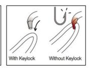
To ensure optimal efficiency, Bm'D carabiners use the Keylock system: the body/gate interface does not have a hook that could snag on anchors, ropes, harness equipment loops...
