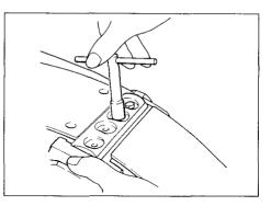
To install the blades, first clean out all chips or foreign matter adhering to the drum or blades. Use blades of the same dimensions and weight, or drum oscillation/vibration will result, causing poor planing action and eventually tool breakdown.
