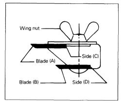
Immerse the dressing stone in water for 2 or 3 minutes before sharpening. Hold the holder so that the blades both contact the dressing stone for simultaneous sharpening at the same angle.
