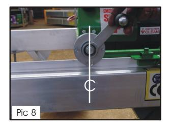
Fit Side Shift Winder assembly (1) into engine frame where trolley roller was removed
