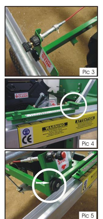
Loosen the Side Shift Brake & remove.
