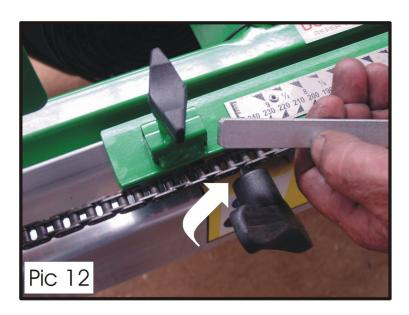
Final position of horizontal ruler gauge, chain & 'T' bolt
