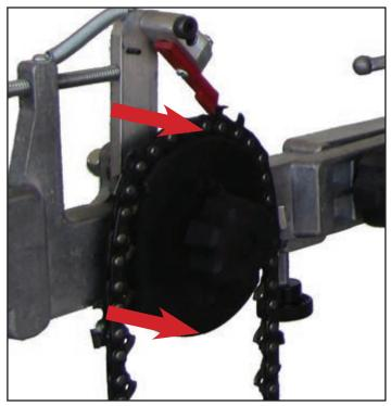
This disk has a .050" groove on one end and a .063" groove on the other. This groove must match the gauge of the drive-links on the chain you intend to sharpen. Adjust the disk so the groove you want is on top and its flat sides tilted a little forward from vertical.
