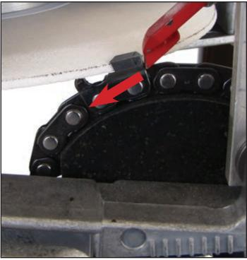
As cutter-teeth become shorter, it is necessary to advance to red stop-pawl to achieve corner alignment. As a consequence, the cutter sits further down the arc, and the inside-top-plate angle becomes more blunt. To compensate for this, the arm holding the chain-guide can be set lower when sharpening chains with short cutter-teeth.
