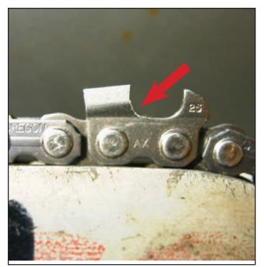
The gullet on this cutter-tooth has been ground out. Gullets can be removed with a round grinder or round file. The Simington #451C does not remove gullets, but they need to be removed for a sharp square-chisel chain to perform well.
