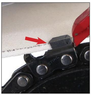
Before you turn the motor on, make sure nothing is touching the grinding wheel. Notice the corner of the wheel is aligned with the outside corner in the cutter-tooth. This is what you need to accomplish.
