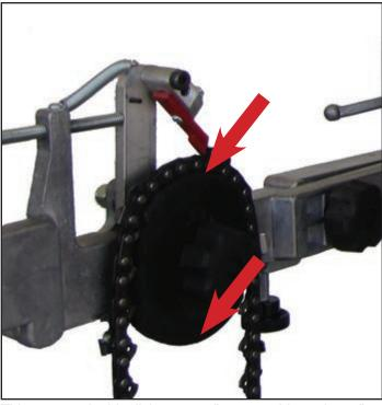
This grooves in this disk are .050" on one side and .063" on the other. Position the groove that matches your chain up. It can tilt slightly forward like this one if you wish. The exact position does not affect the grind angles.
