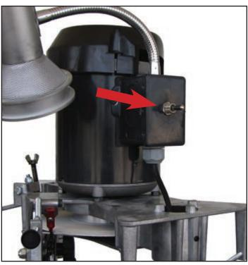
The motor will run in either direction. Pull this switch toward the side you wish to sharpen. This should cause the wheel to rotate into the cutter tooth. The switch has three positions: on-off-on.
