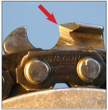
Getting proper corner alignment is the secret to well performing square-chisel saw chain. It is the single biggest factor affecting cutting performance. The corner alignment on this cutter-tooth is perfect.
