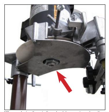
When replacing the grinding wheel, be sure to replace the wheel guard.
