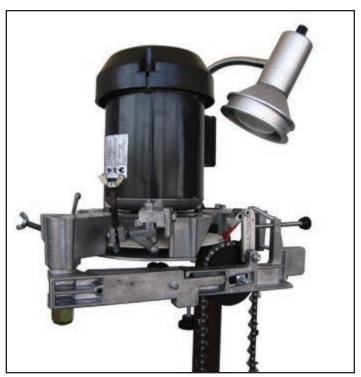
A Simington #451C square-chisel saw-chain grinder mounted on its stand.
