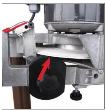
To check if the plane of the wheel matches the sweep of the swing-arm, back off the feed-stops and adjust the arm height so the chain holding disk just fits under the grinding wheel. Then swing the arm over to the other side and measure if there is a difference.
