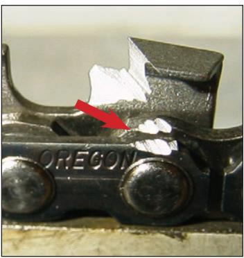
If the edge-thickness of the grinding wheel is too great and/or the grinder is not set up correctly, the chassis of the cutter-teeth can be damaged during sharpening.
