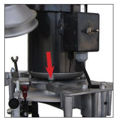
This is one of four motor-mount posts that can be shimmed to match the plane of the wheel to the sweep of the swingarm. These planes need to match or the grinder will not produce similar angles on right-hand and left-hand cutterteeth.
